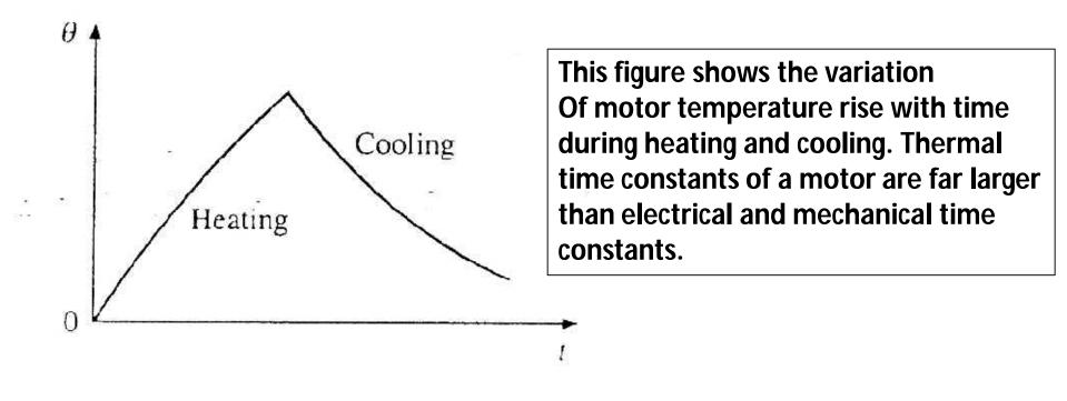
Fig. 5.1. Heating and cooling curves
