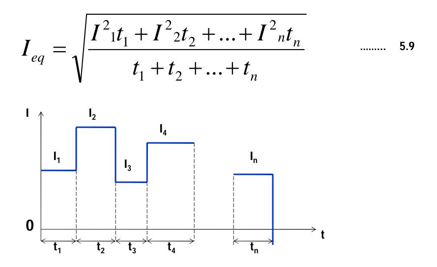
Fig. 5.5. (a) Load diagram of Fluctuating load
