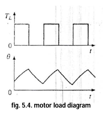
It consists of periodic duty cycles, each consisting of a period of running At a constant load and a rest period. Neither the duration of running period is sufficient to rise the temperature to a Steady value nor the rest period is long enough for the machine to cool to ambient temperature.
