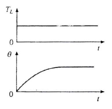
It denotes the motor operation at a constant load torque for s duration long enough for the motor temperature To reach steady state value. This duty is characterized by a constant motor loss.
