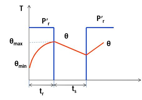
t<sub>r</sub> and t<sub>s</sub> are thermal time constants of motor for working and standstill
