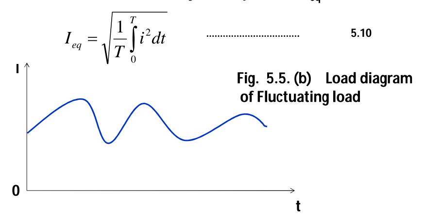
After I<sub>eq</sub> is determined, a motor with next higher current rating from commercially available rating is selected. Then this rating is checked for its practical feasibility . i.e.,
