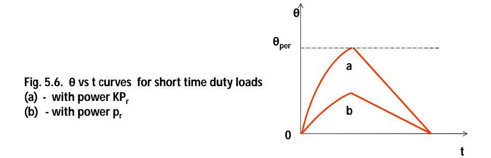
When the duration of running period in a duty cycle with power KP<sub>r</sub> is t<sub>r</sub>, then from equation 5.5;
